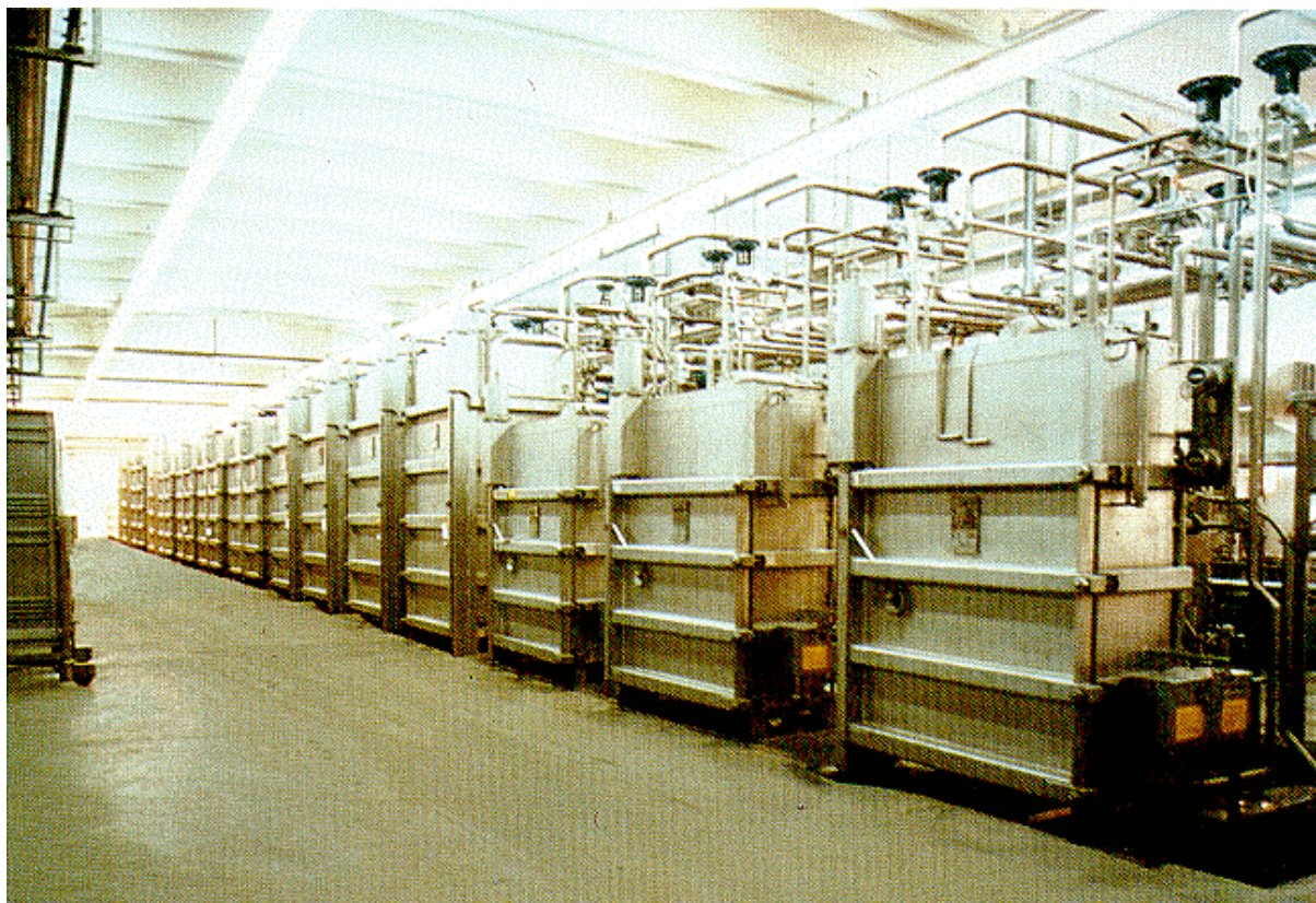
Large automated dyehouse for worsted knitting yarns on hanks. No.22 pressurized cabinets APPC-LV linked to central host computer. Centralized heat recovery system and water recycle by reverse osmosis. VLS variable loading system.
