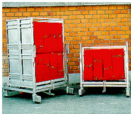
APPC-LV operates at full or half load just by using 1-tier or 2-tier hank loaders.
