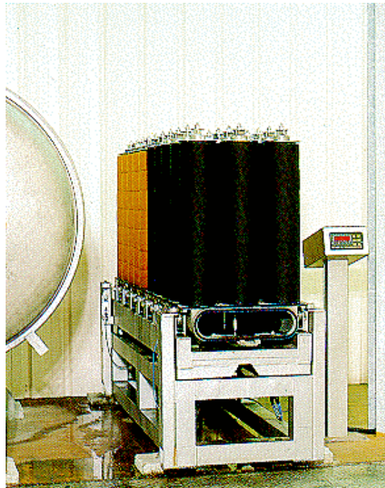
Automated platform for dyeing carrier weighing before drying. Carrier weight is transmitted to calculate the quantity to be removed during drying.
