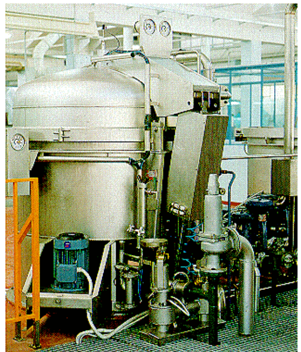
Rear side of TCC with Inverter-driven AC motor, pneumatic lid lifting and automatic valves for liquor drain separation in function of heat recovery.
