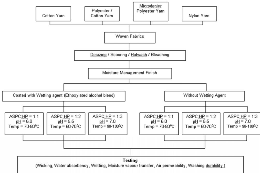
Cotton & Polyester/Cotton blend fabrics were desized, scoured and bleached while Microdenier polyester & Nylon fabrics were hot washed and bleached. After the preparatory processes for four types of fabrics, the following two different techniques were adopted for the development of moisture management finish:
