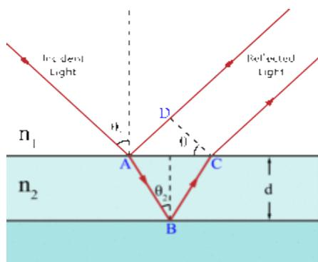
It is the result of interference between reflections from two (or more) surfaces of thin films, combined with refraction as light enters and leaves such films. The geometry then determines that at certain angles, the light reflected from both surfaces adds (interferes constructively), while at other angles, the light subtracts. Different colors therefore appear at
